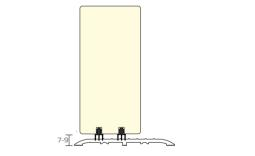
**2.1** The NOR720 should overlap the door stop by 0.5-1mm.
