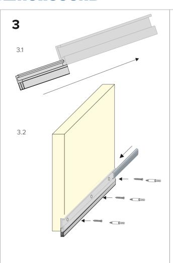
**3.1** Insert the rubber seal into the holder.
