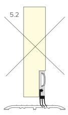
**5.1** The NOR855 can also be surface mounted. NOTE: If surface mounted allow space for the door stops when measuring and cutting the seal.
