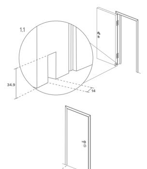
1.1 If installed, remove door from hinges lay on its side and restrain firmly. Using a router machine mortise the bottom of door a groove 34.9 x 14 mm the full width of the door.
