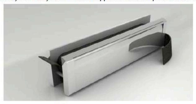
The two halves of the steel letterbox frame are attached by means of steel through-bolts (M4 size) which engage into steel bosses on the opposite frame.
